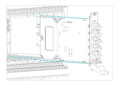
4 Push module into slot until you feel resistance from the backplane connection.
