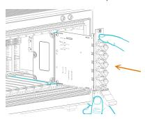
**5** Engage the fastening clip. Secure all fastening screws.
