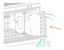
**5** Engage the fastening clip. Secure all fastening screws.
