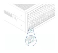
**2** Unsecure the fastening screws and fastening clip.
