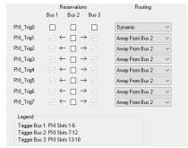
Each slot can create a trigger and the trigger event can be transferred through each PXI Trigger line. Configuring the trigger line can be done easily through NI MAX software interface for the PXIe mainframe.
