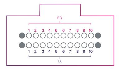
The 1x12 switches are connected to the transceiver using a 24-fiber MPO break-out cable, with each row of 12 fibers connecting to a 1x12 switch. The common ports of the two 1x12 switches are then connected to the input and output of the Variable optical attenuator.
