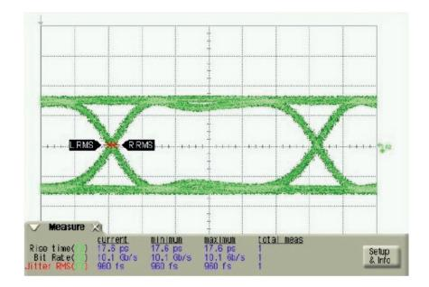
This example shows individual channel cross-test capability of the test system on a single transceiver module, but the setup is scalable. It can easily be configured to cross-test Tx and Rx parts across multiple transceiver modules to identify the point of failure.
