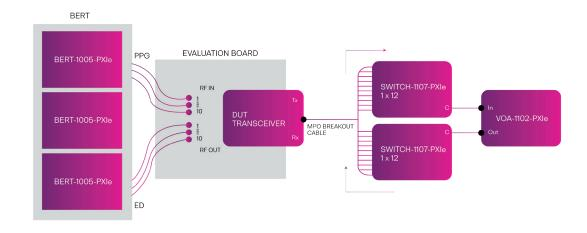
In this simple example, we assume the DUT to be a 100GBase-SR10 pluggable transceiver which uses a 24-fiber MPO for 10 channels of 10Gbps NRZ signal.
