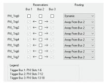
Each slot can create a trigger and the trigger event can be transferred through each PXI Trigger line. Configuring the trigger line can be done easily through NI MAX software interface for the PXIe mainframe.
