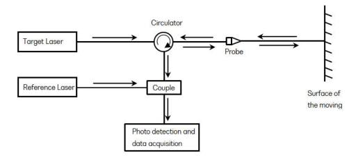
For PDV systems, Quantifi Photonics provides almost all the necessary instruments. The Doppler instruments include components like the circulator and the coupler, and the tunable laser source instrument can be used to generate the target and the reference laser. In addition, you can also use an optical-to-electrical (O2E) instrument to convert the optical signal, which can then be displayed on an oscilloscope.
